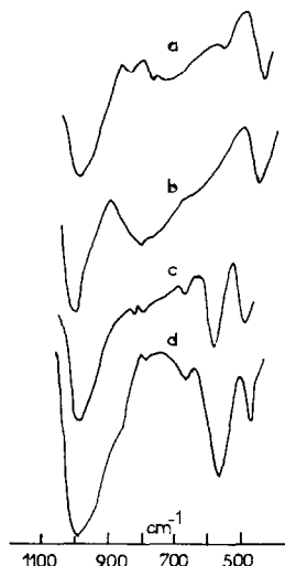
FIG. 7. Infrared spectra of \text{NH}_4\text{A} zeolites treated under hydrolyzing conditions (400 to 1100 \text{cm}^{-1} range). (a) T_4 treatment at 300°C in deep bed; (b) T_4 treatment at 500°C in deep bed; (c) as (b) but with samples initially saturated with water; (d) T_5 treatment followed by T_1 treatment at 500°C under vacuum.
